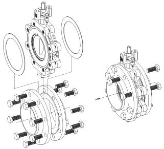
**DANGER:** When installing the butterfly valve with flanged body used in an end-of-line function, the free connection side must be additionally secured by a blind flange or (only for short-term use) the valve must be locked tightly in the "CLOSED" position. The following safety instructions must be heeded:
